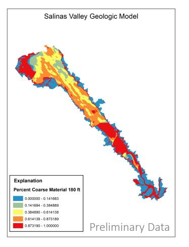
Salinas Valley Geologic Model showing percentage of coarse material distribution for the 180-ft aquifer in the Salinas Valley Integrated Hydrologic Model.
