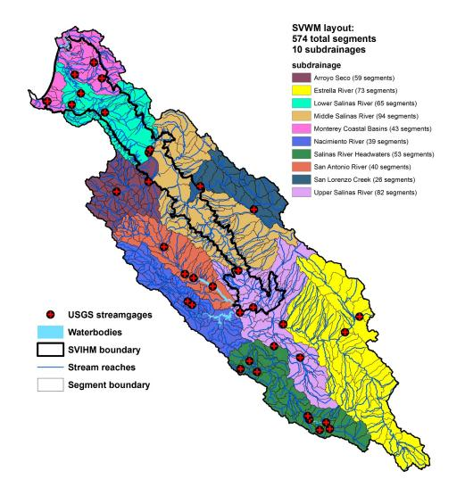
Salinas Valley Watershed Model (SVWM) and Salinas Valley Integrated Hydrologic Model (SVIHM) showing boundaries, stream networks, stream gages, and subdrainages.
