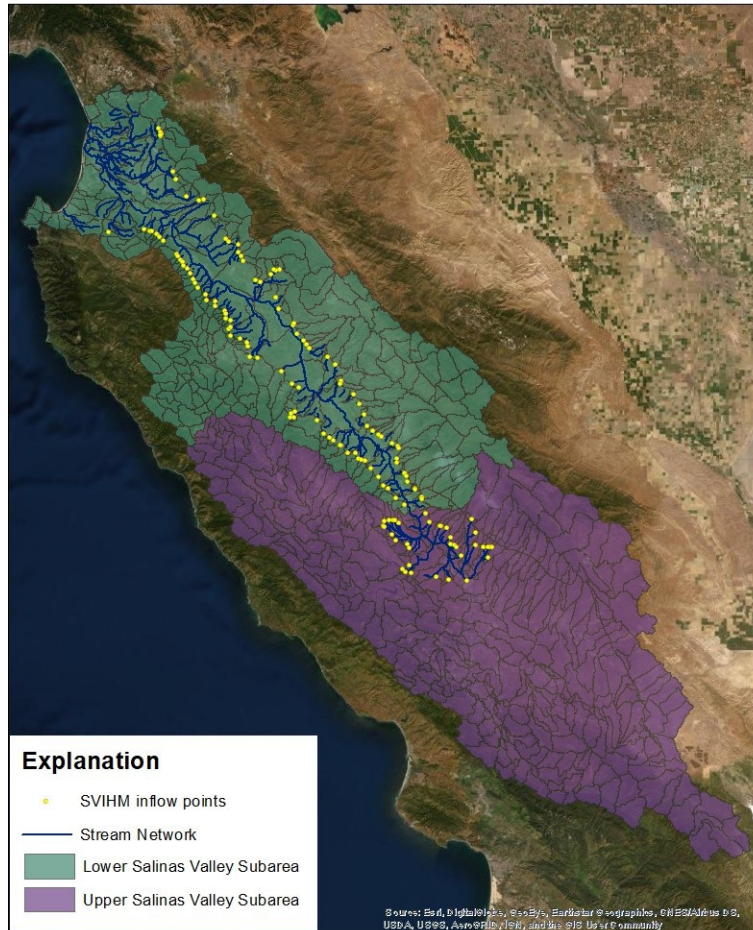
Figure 1: Salinas Valley Watershed Model (SVWM) domain showing Upper and Lower Salinas Valley Subareas, stream network, and inflow points where watershed flows are routed into the Salinas Valley Integrated Hydrologic Model (SVIHM).
