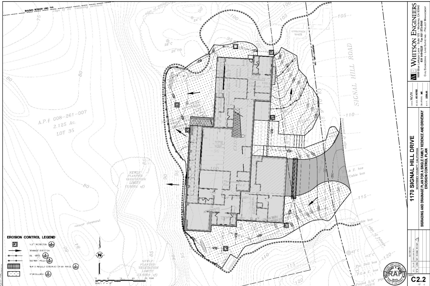
Figure 2-12. Erosion Control Plan
