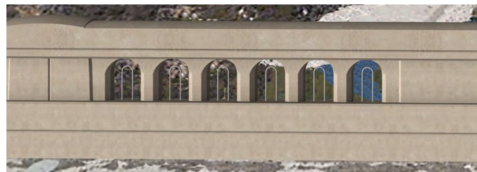
Barrier Alternative - 3D 10" Clear Opening with Dull Galvanized "U" Bar and Chamfered Balusters
