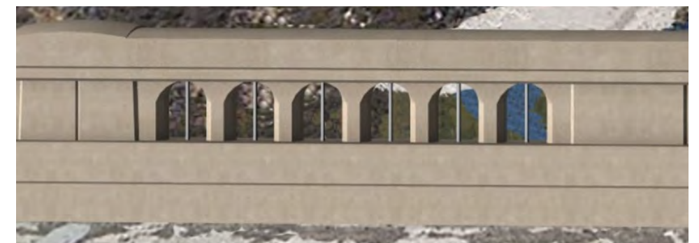
Barrier Alternative - 4D 10" Clear Opening with Dull Galvanized Single Bar and Chamfered Balusters
