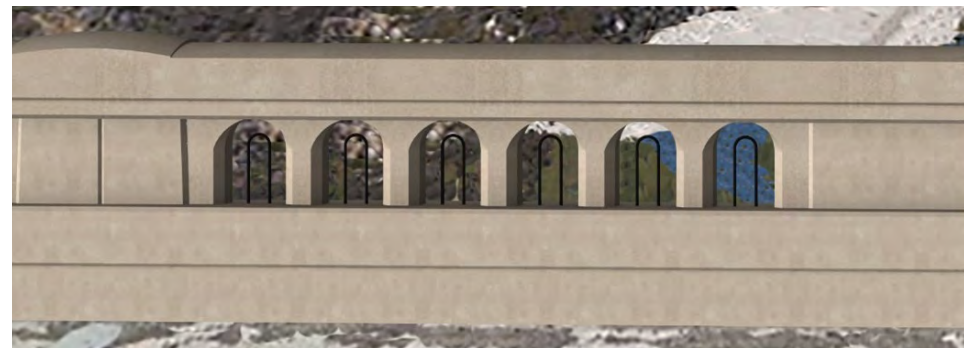
Barrier Alternative - 3C 10" Clear Opening with Dark "U" Bar and Chamfered Balusters
