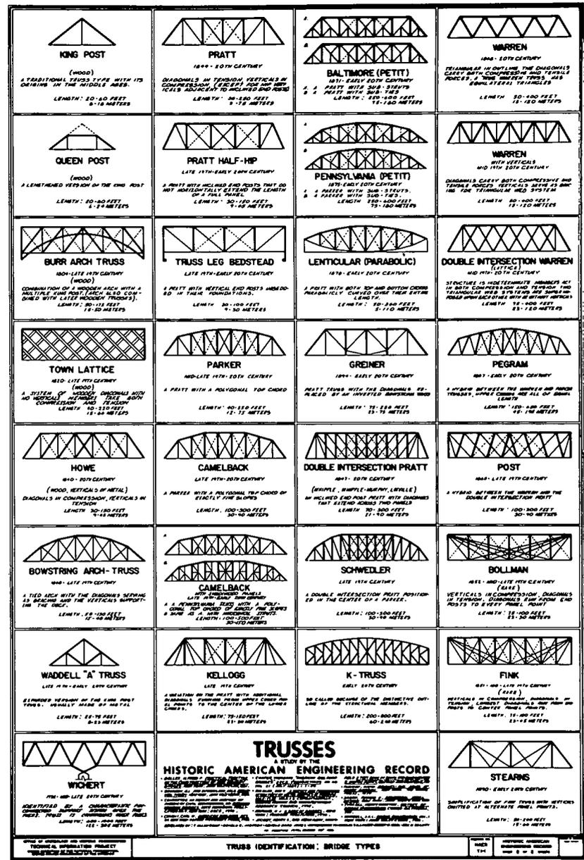
FIGURE 4 Explanation of bridge truss types (HAER).
