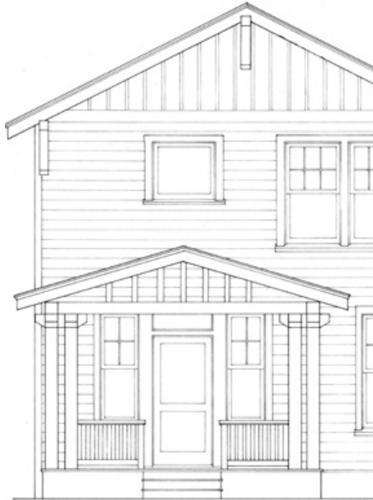
One-story gable-end porch
