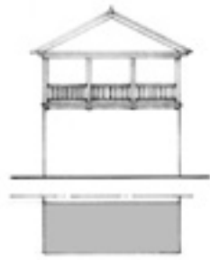
A Two-Story Front Gable with Second-Story Balcony
