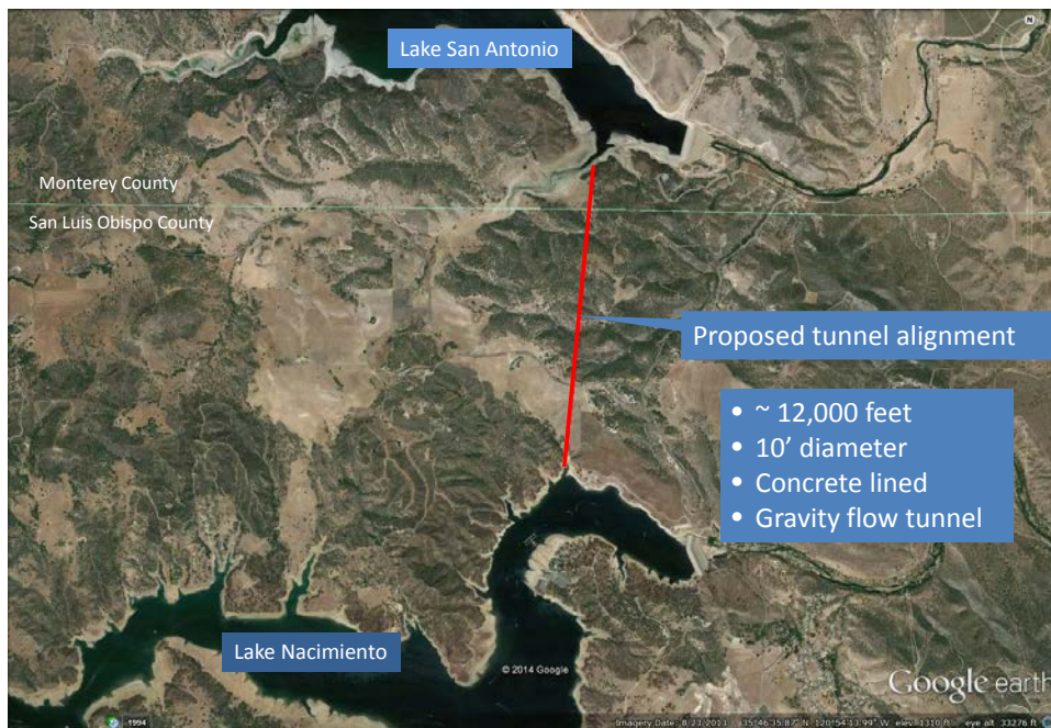
Figure 2 - Interlake Tunnel project description
