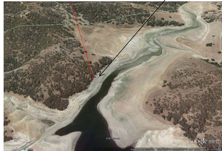
Portal Elevation (TBD) Spillway elevation ~ 780'
