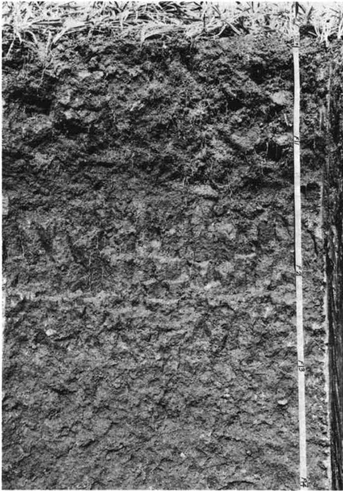
Figure 3.—A typical profile of Danville sandy clay loam, 0 to 2 percent slopes. The clay subsoil is at a depth of 18 inches.
