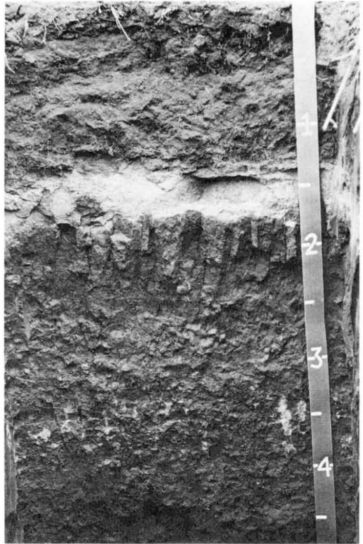
Figure 1.—A typical profile of Antioch very fine sandy loam, 0 to 2 percent slopes.
