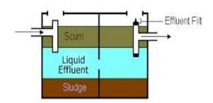
of the system will determine how often the tank should be pumped. Washing machines, dishwashers, and garbage disposals will increase the amount of sludge, and the tank will require more frequent pumping.
