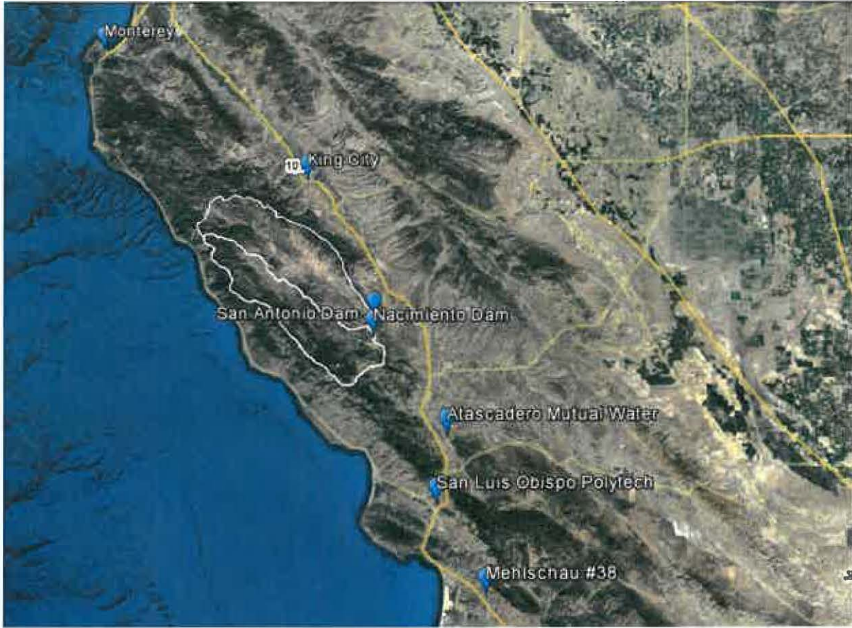
Figure 6.1 Precipitation gauges (blue markers) used in the development of regression equations with the streamflow data; watersheds outlined in white
