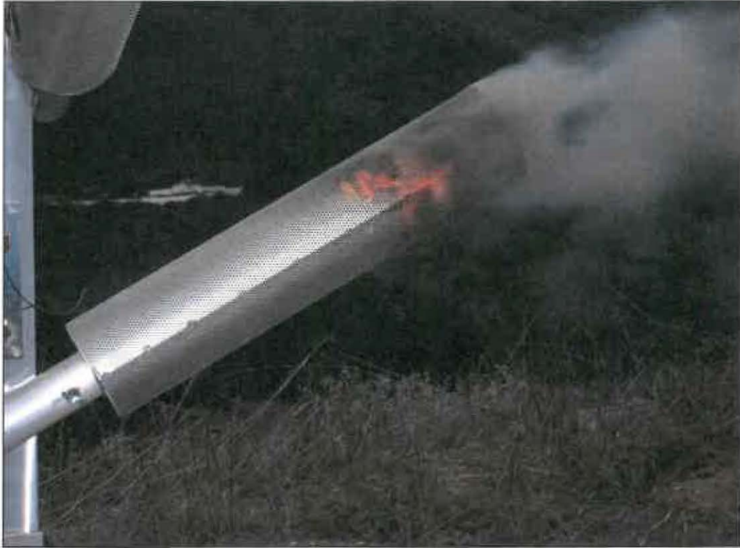
Figure 5.7 Flare Burning Inside Spark Arrestor
