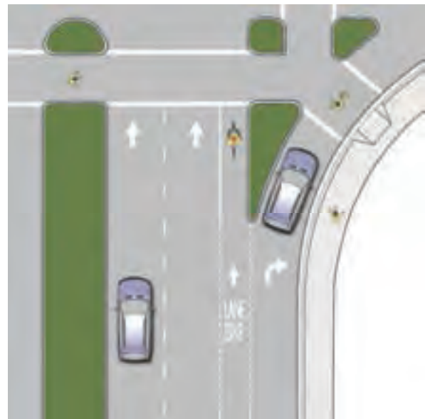
Bike Lane Next to a Right Turn Only Lane Separated by a Raised Island
