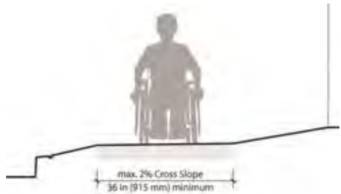
Sidewalk cross slope should not exceed 2% to comply with ADA accessibility standards.
