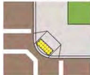
Diagonal Curb Ramp
